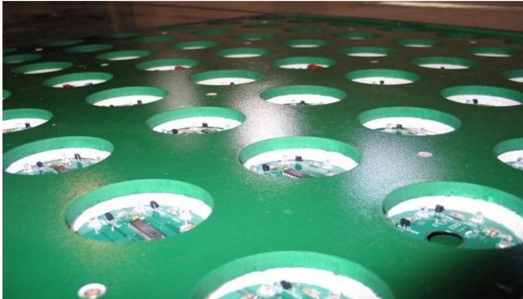
Figure 3: Prototype of Electronic layer for solar roadway
